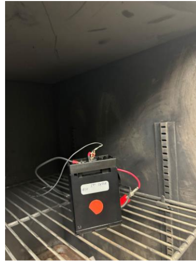
Figure B-8: Sample during Overcharge (T7)
