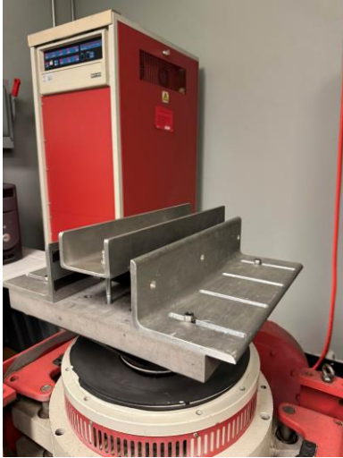
Figure B-3: Samples on the Vibration Table (T3)
