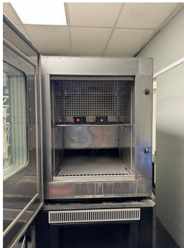
Figure B-2: Samples in the Environmental Chamber (T2)
