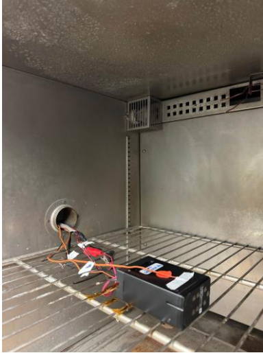
Figure B-7: Sample during Short Circuit Test (T5)
