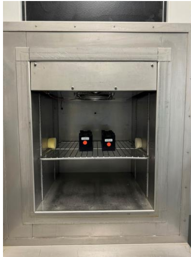
Figure B-1: Samples in the Altitude Chamber (T1)
